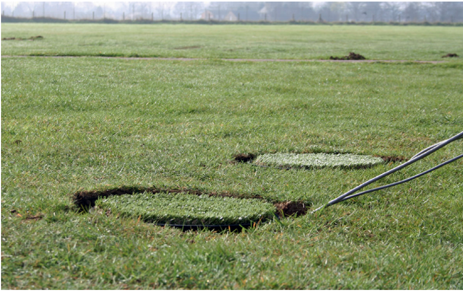
FIG. 3. Two dewmeters with artificial canopies deployed at Cardington. The round canopies can be seen flush with the surrounding grass surface.
