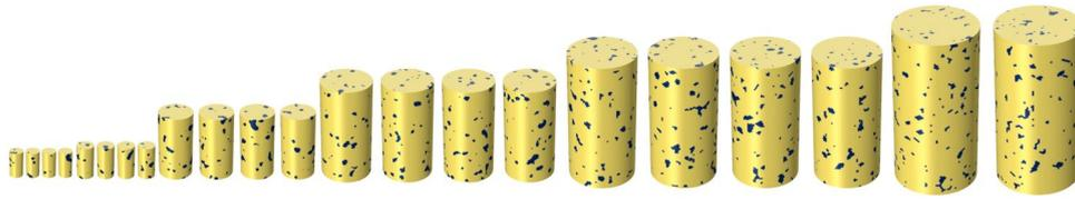
**Fig. 13** Virtual sampling of cylindrical specimens with a slenderness ratio of 2 from the block in Fig. 2. From left to right, four specimens are cored having the diameters of  $4a$ ,  $5a$ ,  $10a$ ,  $15a$ ,  $20a$  and two specimens of diameter  $25a$ , with  $a$  the characteristic size of the heterogeneities
