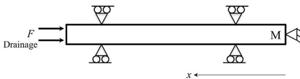
**Fig. 7.** Schematic representation of Terzaghi's problem. The monitoring point ( $M$ ) for Figs. 8, 9 and 11 is displayed.
