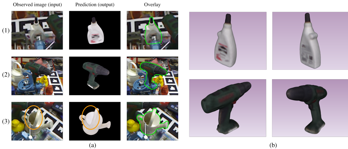
Figure 5-8: Predictions using low-fidelity CAD models. In (a) we show the result of our approach on LineMOD Occlusion for three different objects which have only low-fidelity CAD models available. In (1) and (2), the quality of the mesh and textures is poor as illustrated in (b). Notice for example how the annotations on the glue box or the brand of the drill are not readable on the CAD models. In (3), the hole of the watering can does not appear in the CAD model. Despite these discrepancies between the real object and the CAD model, our approach correctly estimates the pose of each object.
