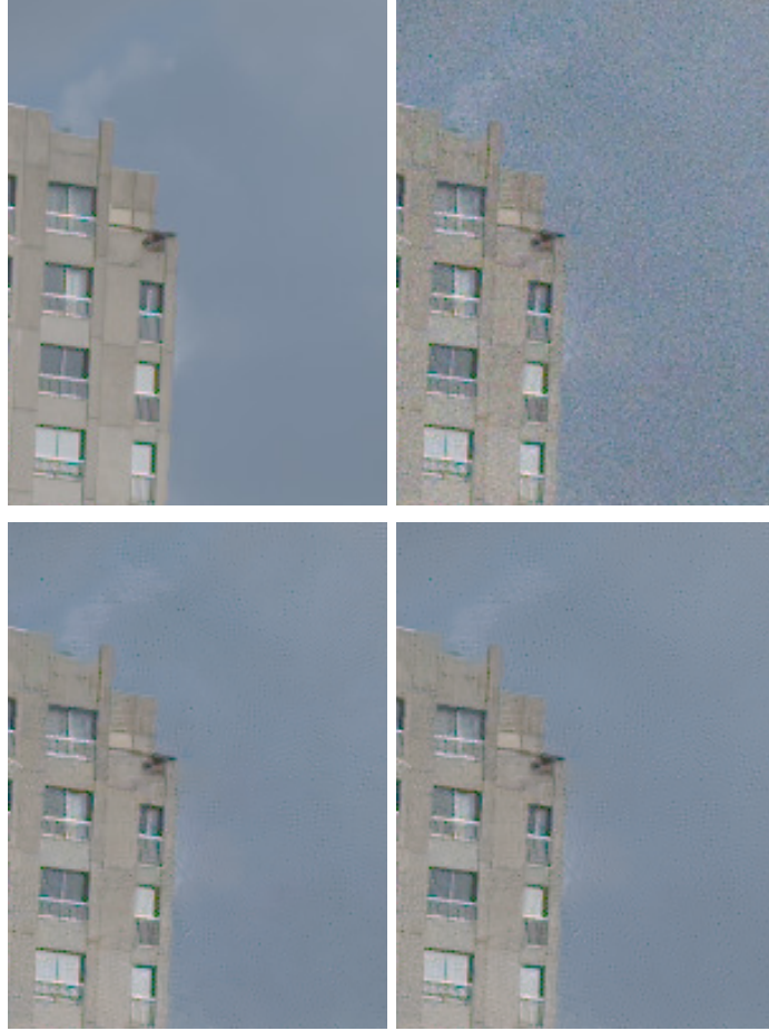
FIGURE 9. Visual results of the JPEG (third) experiment. From top to bottom, and left to right: crop of the noise-free image u_{\text{jpeg}} , crop of the noisy image \tilde{u}_{\text{jpeg}} , crop of the result of the Noise Clinic using two scales \hat{u}_{\text{jpeg}}|^{s^2} and crop of the result of the Noise Clinic using three scales \hat{u}_{\text{jpeg}}|^{s^3} .
