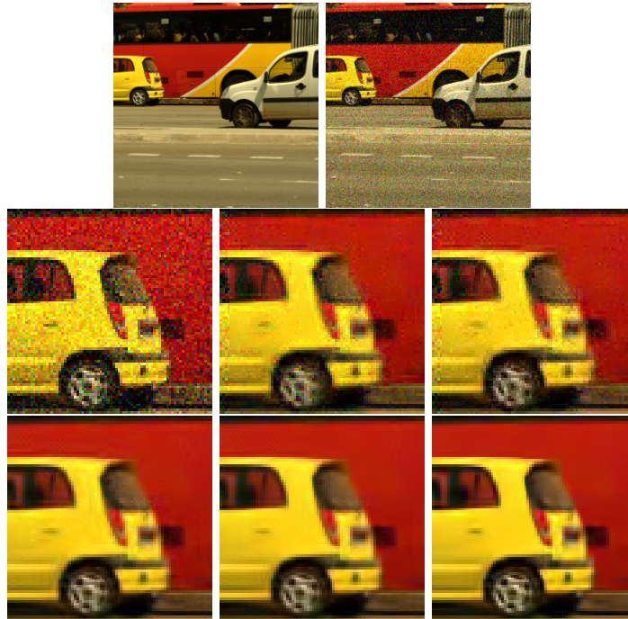
FIGURE 1. Top: original and noisy images with an additive Gaussian white noise of standard deviation 25. Below, from top to bottom and left to right: crop of denoised images by sliding DCT thresholding filter and incrementally adding use of a Y_oU_oV_o color system, uniform aggregation, variance based aggregation and iteration with the “oracle” given by the first step. The corresponding PSNR are 26.85, 27.33, 30.65, 30.73, 31.25.
