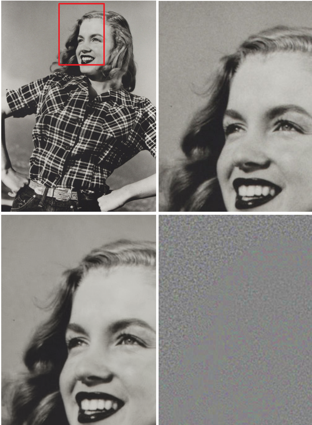
FIGURE 17. Blind denoising on “Marilyn”, using two scales. From left to right, top to bottom : input noisy image, crop of the noisy image, crop of the output denoised image, crop of the difference image.
