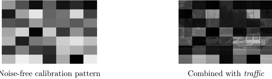
FIGURE 2. On the left, synthetic noise-free calibration pattern. On the right, the weighted sum of the calibration pattern with the noise-free test image traffic (with weights 0.8 for the calibration pattern and 0.2 for the traffic image). Since both combined images are noise-free, the result is still noise-free, but textured.
