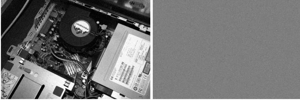
FIGURE 2. Left: Noise-free test image computer (see Section 1 of Chapter 13) after adding homoscedastic white Gaussian noise of \sigma = 10 . Right: pure homoscedastic white Gaussian noise of \sigma = 10 image. Both images have the same 704 \times 469 size.
