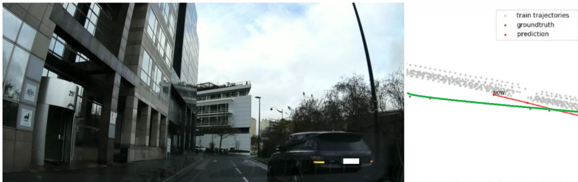
Figure 5.1: Localization failure during an overtaking. Absolute Pose Regression fails to recover the vehicle position in the left lane because this situation requires to extrapolate outside of the training dataset positions.
