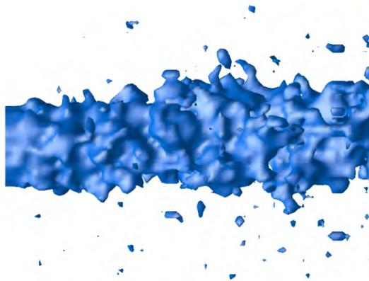
FIGURE 2.19. – Jet diesel en VOF, Bianchi et al. [23].
