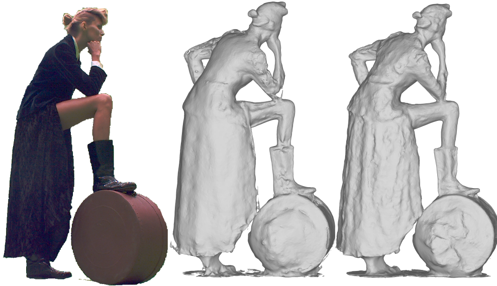
FIGURE 2.5 – Challenging scene captured with a passive RGB multi-camera setup [kin]. (left) one input image, (center) reconstructions obtained with classical 2D features [LFB17], (right) proposed solution. Our results validate the key improvement of a CNN-learned disparity to MVS for performance capture scenarios. Results particularly improve in noisy, very low contrast and low textured regions such as the arm, the leg or even the black skirt folds.
