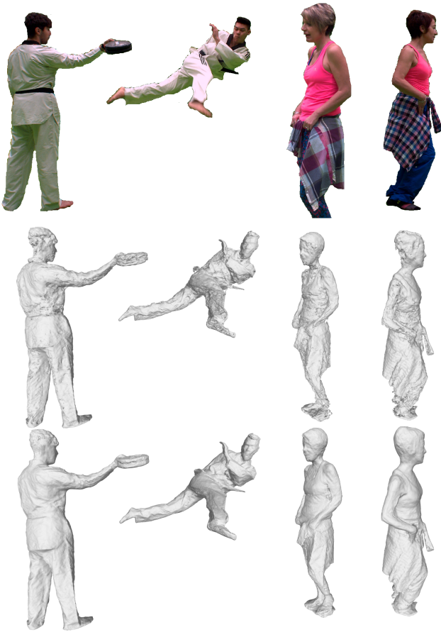
Fig. 13 (top row) Input images of captured subjects. (middle row) Reconstructions without probability accumulation along rays. (bottom row) Results with accumulation.
