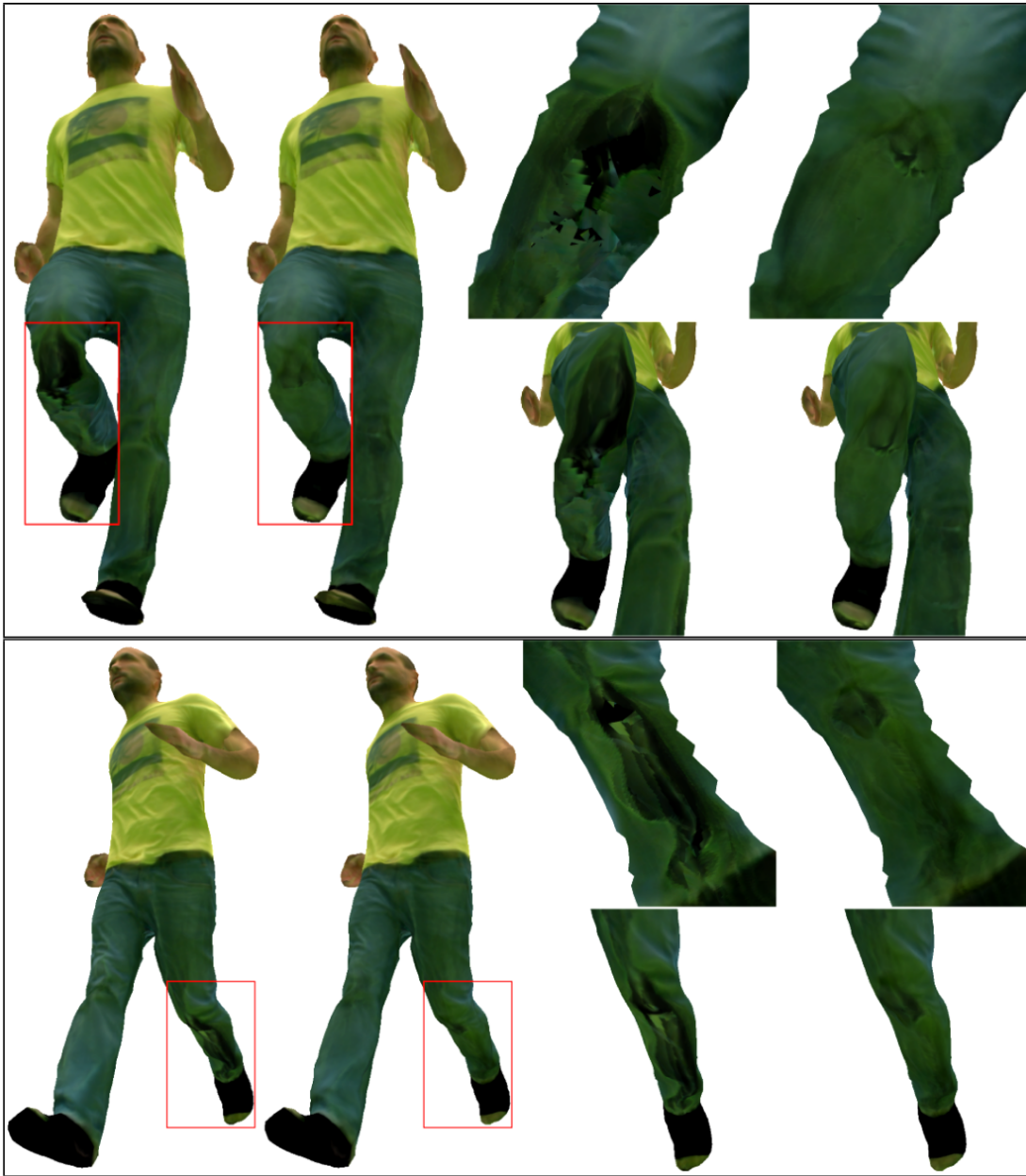
FIGURE 4.8 – Completion examples. From left to right : Input and completed models, close-up on input and completed texture maps (top) and rendered images (bottom).
