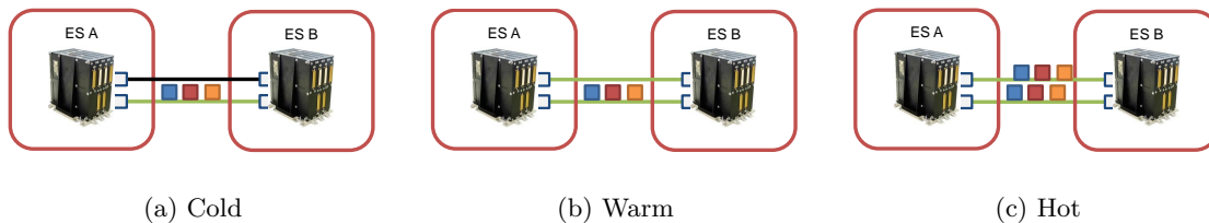
Figure 3.5: Link Redundancy Modes Example
