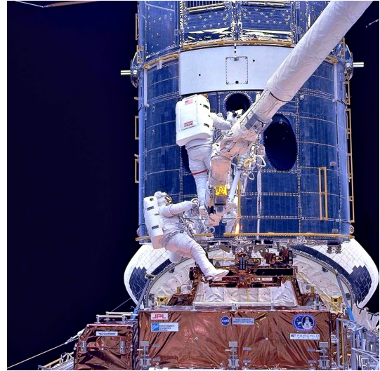
Figure 1.2 – Astronauts Musgrave and Hoffman install corrective optics during the first servicing mission of HST (credits: NASA)
