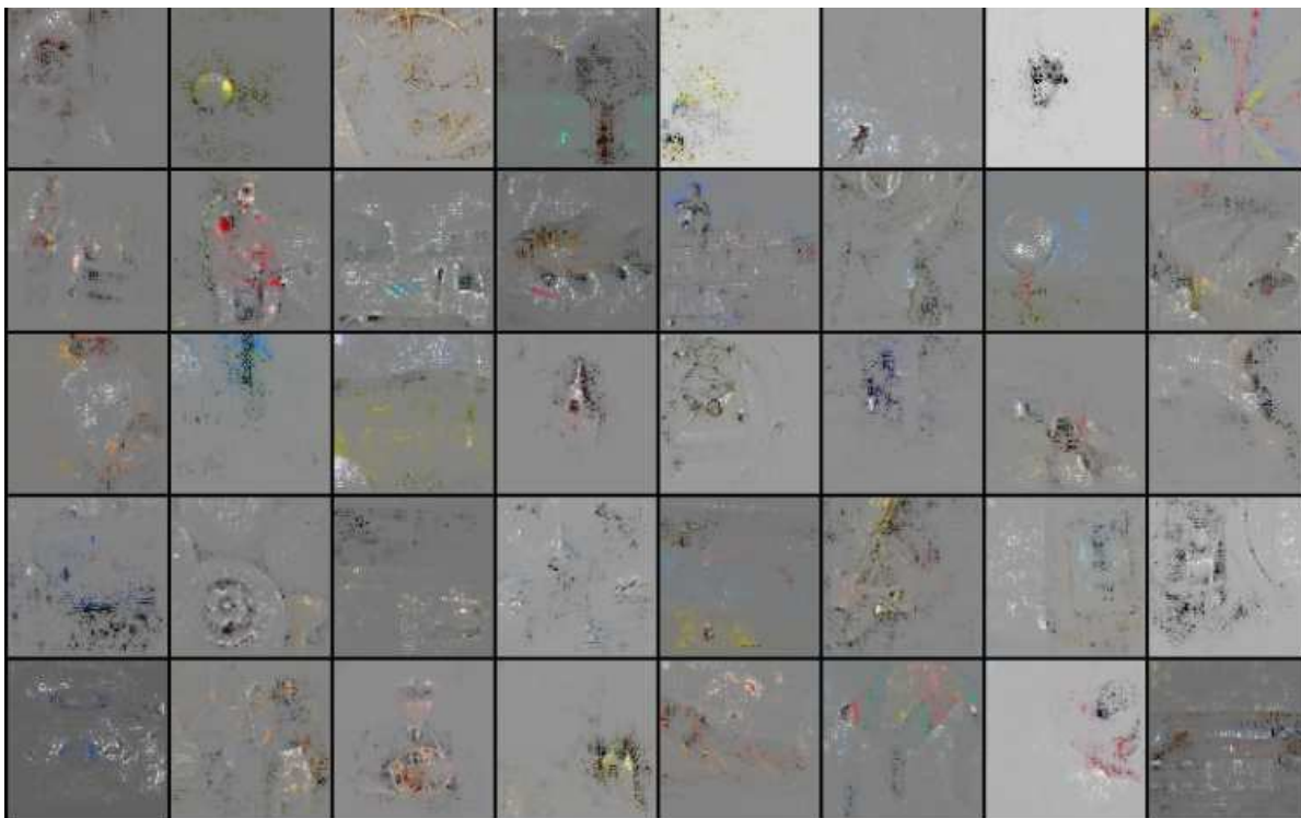
Figure 8.4: Gradient of the loss wrt the input on the current batch. The per-pixel norm of the gradient weighs each pixel's intensity. This helps figuring out what the model looks at in the picture in order to make its predictions
