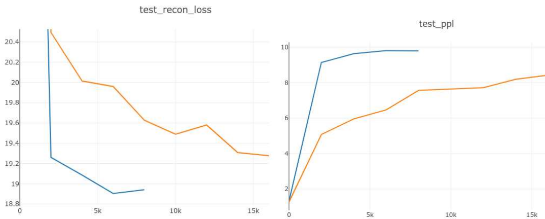
Figure 6.21: Experiment comparing test loss (left) and codebook usage PPL (right) for a codebook of 32 code points. Horizontal axis: training iterations, blue: VQ with expiration, orange: VQ without expiration.
