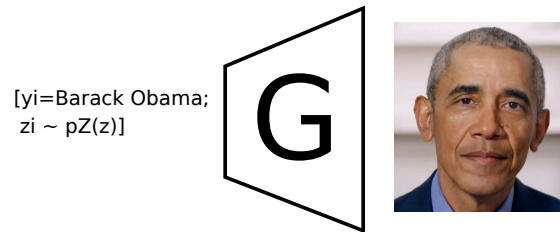
Figure 6.1: G is a generator that turns a person identifier y_i and a latent variable z_i into an image.
