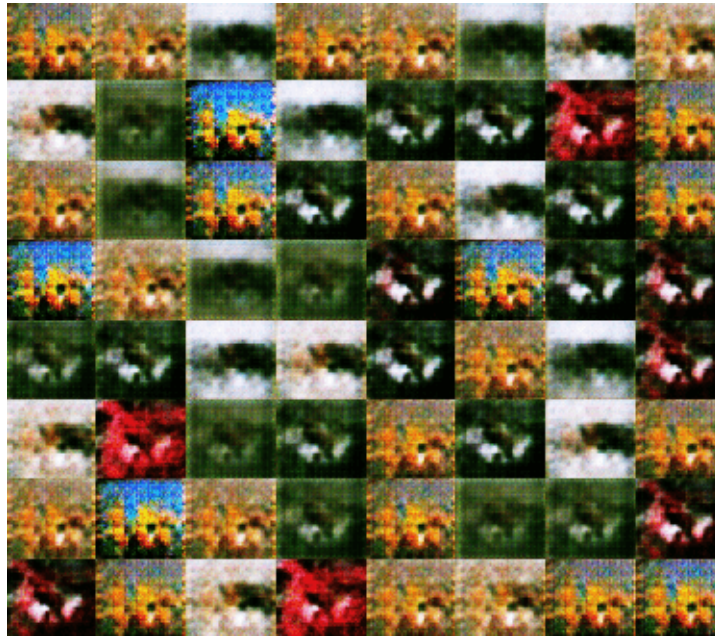
Figure 6.10: An example of GAN training collapse. The generated samples suddenly ceases converging towards realistic samples, and the GAN never escapes this degenerate state. Image source: https://www.mathworks.com/help/deeplearning/ug/monitor-gan-training-progress-and-identify-common-failure-modes.html
