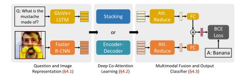
Figure 2.11. – Architecture of MCAN, by Yu et al. 2019. After the image and text embeddings using an LSTM and a Faster R-CNN, a series transformer block with cross-attention is used to merge the image and question representations.
