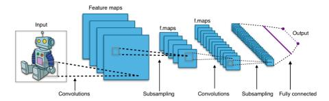
Figure 2.1. – A typical convolutional neural network architecture. It is composed of multiple convolution layers, that match local patterns, pooling layers that reduce the spatial dimension of the feature maps, and fully connected layers at the end, to return a classification output. Image from https://en.wikipedia.org/wiki/Convolutional\_neural\_network
