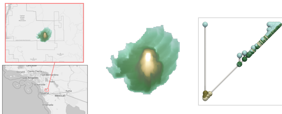
Figure 6.2 – Example of a dataset from the wildfire use case. From left to right: localization of the fire (California), the corresponding scalar field (time of arrival of the fire), and the associated persistence diagram.
