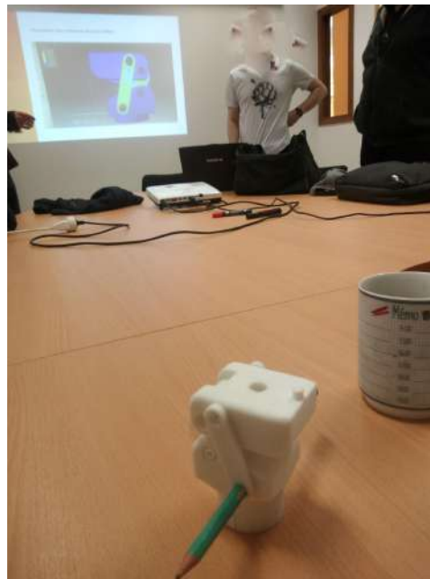
Figure 10.6: Design and 3D printing of a Polycentric Prosthetic Knee Joint
