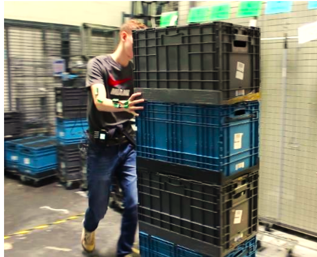
Figure 1.8: Goniometers placed at wrist and elbows levels during the goods reception activity (extracted from Varraut, 2018).
