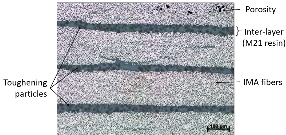
Figure 2.2: Micrograph through the thickness of an IMA/M21 laminate cured sample.
