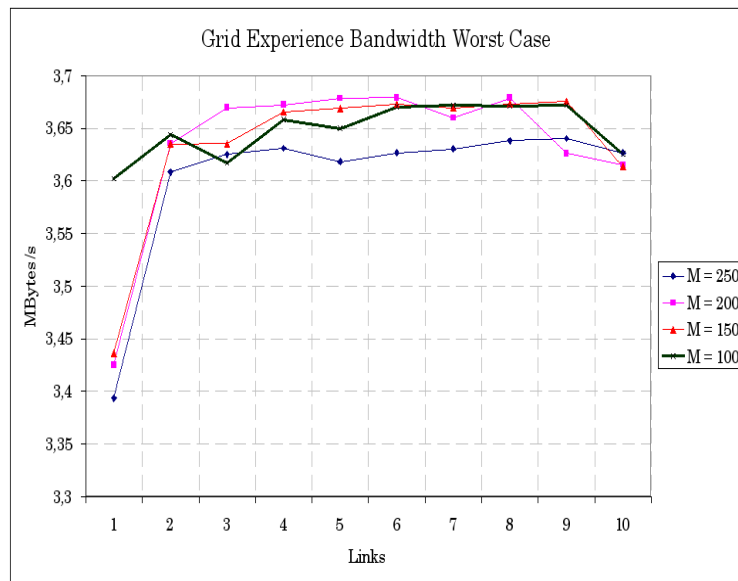
Figure 5.30: GDX-Grillon Transfer: Bandwidth Worst Case Measurement
