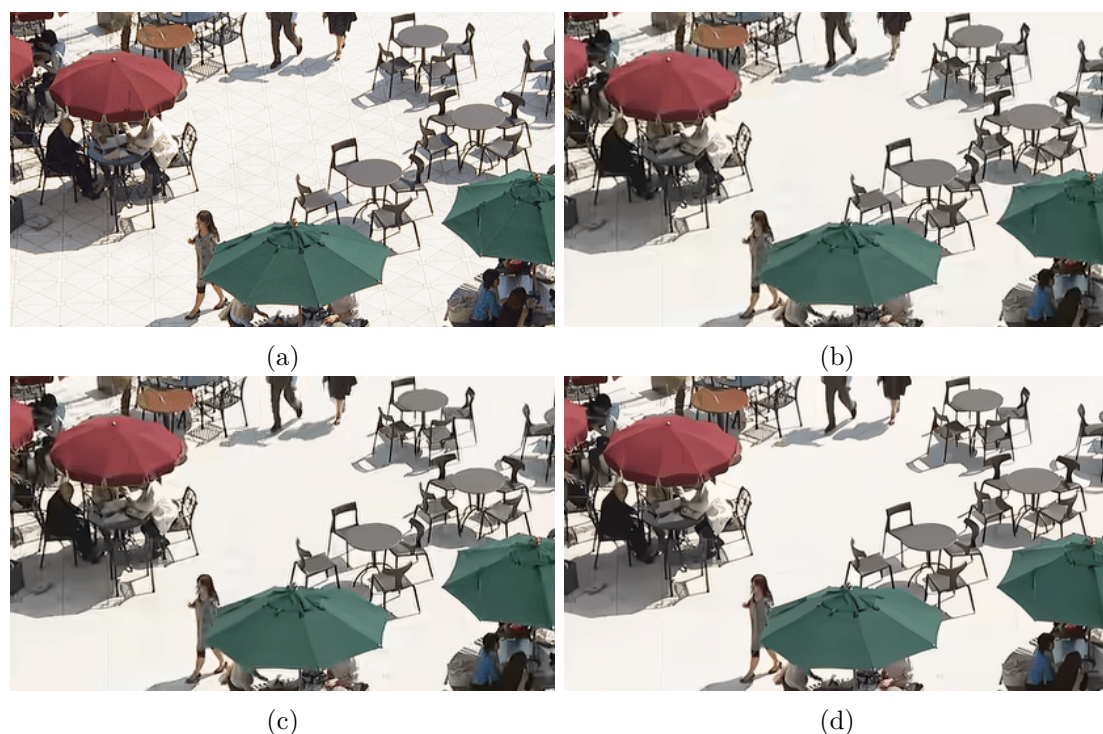
Figure. III.7: Ablation Study. Subjective Visual Quality Comparison (the 12th frame of BQSquare with QP=37 ): (a) Original; (b) VVC without in-loop filtering ( PSNR=31.17\text{dB} ); (c) VVC ( PSNR=31.37\text{dB} ); (d) VVC-based proposed model ( PSNR=31.68\text{dB} )
