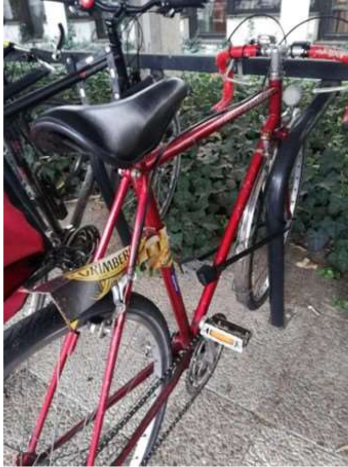
Figure 3.5 - Cardboard from a beer pack turned into a DIY mudguard
