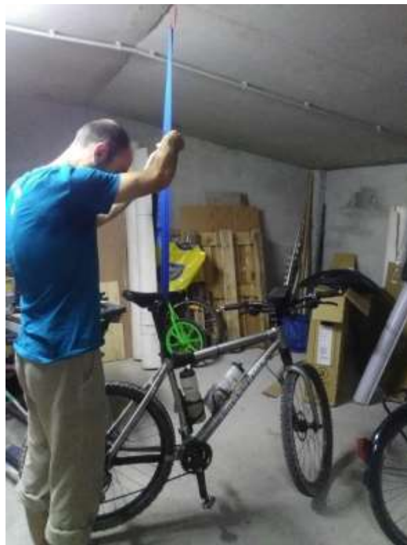
Figure 2.9 - Home-made solution to keep a cycle still for maintenance and repair
