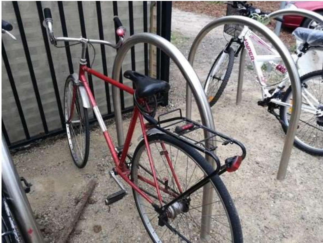
Figure 3.4 - A cycle with inverted handlebars, a transformation sometimes adopted by cyclists wishing to ride with a more upright posture than the one encouraged by the initial position of the handlebars
