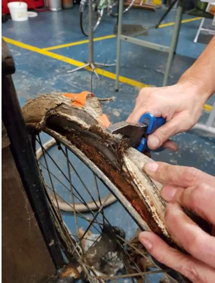
Figure 0.4 - Breaking the threads of a very old tyre in order to extract the inner tube from the wheel, Lyon
