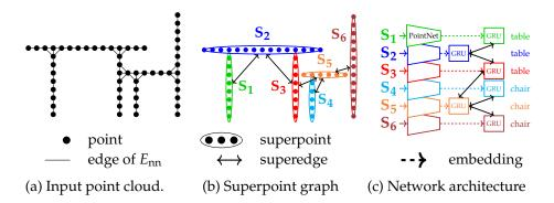
Figure 3.4: **Pipeline.** We illustrate our approach on a toy scene with a table and a chair. We partition the point cloud (a), which allows us to build the superpoint graph (b). Each superpoint is embedded with a PointNet network. The embeddings are then refined with message passing along superedges to produce the final labelling (c).
