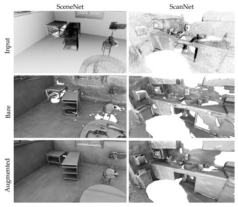
Figure 4.12: **Out-of-Domain Scene-Level Reconstruction.** POCO trained on ModelNet10, with and without visibility information, is run on scenes from SceneNet (synthetic RGB-D scan) and ScanNet (real RGB-D scan).
