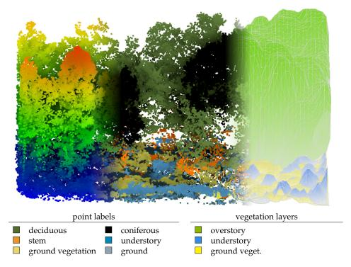
Figure 4.14: **Multi-Layer Forest Analysis.** We introduce WildForest3D, a novel dataset of annotated UAV-LS point clouds of dense forest (left), and a new model for the multi-layer analysis of vegetation. Our network performs 3D semantic segmentation (middle), and produces height maps and watertight meshes for three vegetation layers (right).
