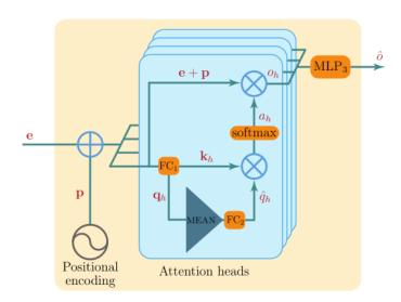
Figure 5.4: **Architecture of the Temporal Attention Encoder.** Our simplified transformer architecture can efficiently embed sequences of image embeddings. Variables in bold are tensors concatenated along the temporal dimension, e.g.  $\mathbf{e} = [e^{(0)}, \cdots, e^{(T)}].$
