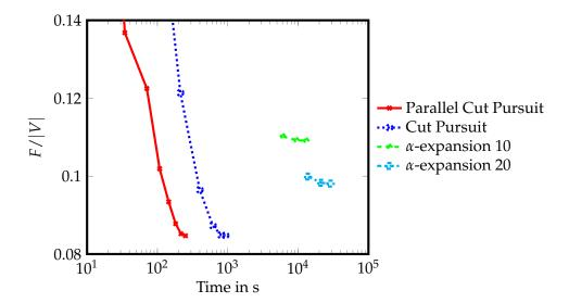
Figure 2.7: **Numerical Experiment for**  $\ell_0$ -**cut pursuit.** We represent the evolution of F/|V| with respect to computation time in seconds. The cut pursuit algorithm produces its approximation in little more than 2 minutes with parallelization, and under 7 minutes without. In contrast,  $\alpha$ -expansion takes up between 2 and 8 hours depending on the chosen number of labels and desired precision.
