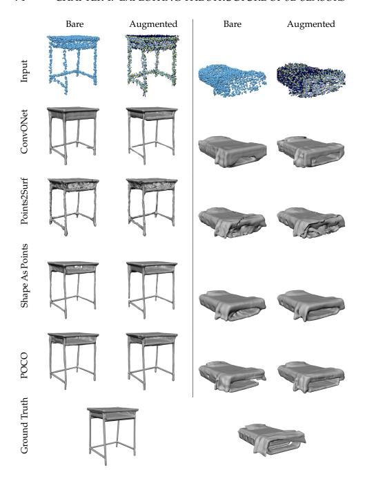
Figure 4.11: **Object-Level Reconstruction.** Shapes from the ModelNet10 test set reconstructed using four different DSR methods operating on point clouds with and without our proposed visibility-augmentation.
