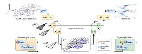
Figure 4.3: **Helix4D Architecture.** A point sequence is split into angular slices and encoded with a cylindrical convolutional encoder  $\mathcal{E}^{\mathsf{grid}}$ . At the lowest resolution, we apply W consecutive spatio-temporal transformer blocks  $\mathcal{T}^w$  with attention spanning current and past slices. The resulting features are up-sampled to full resolution with a convolutional decoder  $\mathcal{D}^{\mathsf{grid}}$  and used to classify the individual points.
