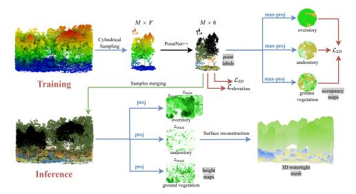
Figure 4.15: **Multi-Layer Modeling.** Our network yields label predictions for each 3D point, which are projected onto rasters to obtain soft occupancy maps for 3 different vegetation layers. The network is supervised using 2D and 3D annotations. During inference, the predictions are used to derive the minimum and maximum elevation of each layer, which we convert in a watertight 3D mesh.
