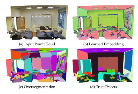
Figure 3.5: Learning to Partition. We process a point cloud (a) with our point embedding network (b). We compute a piecewise constant partition of these embeddings (c), which closely follows the ground truth objects (d).
