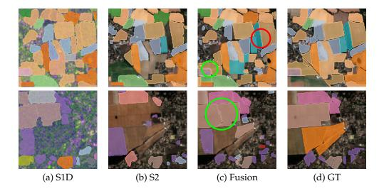
Figure 5.16: **Qualitative Results for Panoptic Segmentation.** We compare the predictions made by unimodal models operating on S1D (a), S2 (b), the late fusion model (c), and the ground truth annotations (d). Some parcels are misclassified when only using the optical modality but are successfully recovered by the radar and fusion models (green circle  $\bigcirc$ ). Some parcels are only detected using both modalities (red circle  $\bigcirc$ ).
