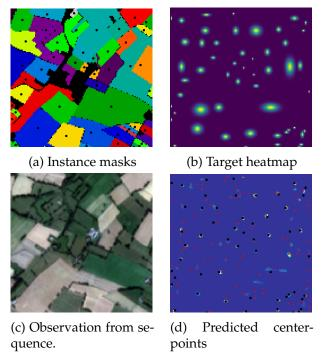
Figure 5.10: **Centerpoint Detection.** The ground truth instance masks (a) is used to construct a target heatmap (b). Our parcel detection module maps the observation (c) to a predicted heatmap (d). The predicted centerpoints (red crosses) are the local maxima of the predicted heatmap (d). The black dots are the true parcel centers.
