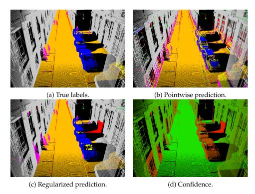
Figure 3.1: **Smoothing a Pointwise Prediction.**:A 3D point cloud taken from the Paris-rue-Cassette Dataset [VBS<sup>+</sup>15] and with true annotation (a). A pointwise classifier first gives a noisy semantic segmentation (b) which we smooth to improve the spatial regularity (c). Our approach allows to retain the probabilistic nature of the segmentation (d): confident uncertain. Note that misclassifications in (c) correspond to the least confident area in (d).
