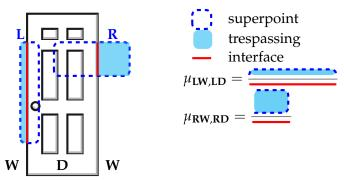
Figure 3.7: Cross-Partition Weighting. Scene comprised of a door (D) and a wall (W). Two superpoints L (left) and R (right) overlap the door. The edges of (LW,LD) (resp. (RW,RD)) connect the vertices of the left (resp. right) superpoint that belong to the wall and the door. With fewer trespassing vertices and a longer interface than (RW,RD), the weights of (LW,LD) are smaller.
