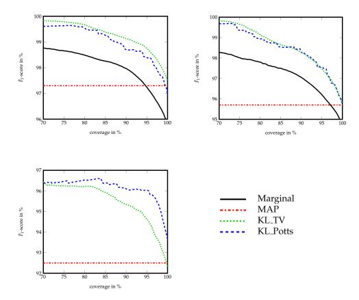
Figure 3.2: **Quantitative Results for Label Smoothing.** Accuracy/coverage plot: we sort the points by decreasing confidence for the Oakland-3C dataset (top left), the Oakland-5C dataset (top right) and the Paris-rue-Cassette database (bottom left). The precision reaches nearly 100% for probabilistic methods at coverage 70%, *i.e.* once removing the 30% least confident points
