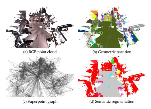
Figure 3.3: **Superpoint Graph.** An input point cloud (a) is divided into geometrically simple shapes, called superpoints (b). We construct a graph by linking nearby superpoints with superedges (c). We then use graph convolutions to classify the superpoints according to their shape and context.
