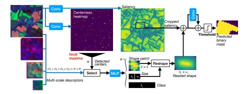
Figure 5.11: **Panoptic Segmentation.** The local maxima of the predicted centerness heatmap define M tentative parcels. We then predict a bounding box size, a semantic class, and an  $S \times S$  shape patch for each detected centerpoint. Combined with a global saliency map, the shape patch allows us to predict pixel-precise masks.
