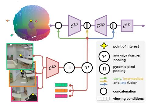
Figure 4.6: **Bimodal 2D/3D Architecture.** We combine a 2D convolutional encoder  $\mathcal{E}^{\text{2D}}$  and a 3D network composed of an encoder  $\mathcal{E}^{\text{3D}}$ , a decoder  $\mathcal{D}^{\text{3D}}$ , and a classifier  $\mathcal{C}^{\text{3D}}$  with three different 2D/3D fusion strategies: early (our choice in the experiments), intermediate, and late fusion.
