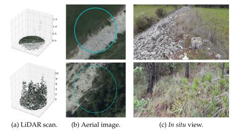
Figure 4.17: **Plot-Based Annotations.** We represent in (a) the 3D point clouds corresponding to two distinct plots. In (b), we show an aerial view of the plots, and in (c) the perspective of the  $in \, situ$  annotator. The top plots has a layer coverage of 0%, 10%, 50% for overstory, understory, ground vegetation, and the bottom plot 40%, 60%, 50%.
