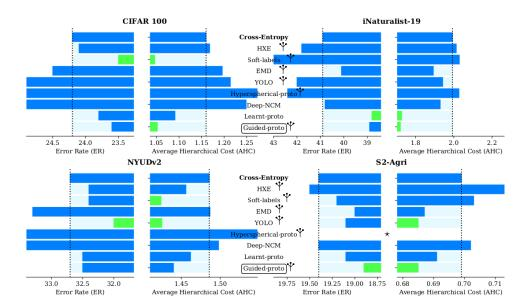
Figure 5.20: **Quantitative Results.** Error Rate (ER) in % and Average Hierarchical Cost (AHC) on four datasets for Guided-proto, the Linear Classifier baseline (Cross-Entropy), and competing approaches. Methods that use the hierarchical knowledge are indicated with the symbol \*. We plot the best performances on each dataset in green. Our guided prototype approach improves the ER and AHC across the four datasets compared to the baseline. \*: would not meaningfully converge.
