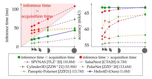
Figure 4.4: **Influence of Slice Size.** We plot the processing time (left, in ms) and precision (right, in mIoU) of different methods for the considered slices sizes, estimated on the validation set of SemanticKITTI [BGM<sup>+</sup>19]. Methods whose inference time is slower than the acquisition time of the slice (red shaded area) do not meet the real-time requirement.
