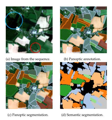
Figure 5.8: **Problem Statement.** We consider an image sequence (a) with panoptic annotations (b). Our objective is to learn spatio-temporal pixel features, which can be used to perform panoptic (c) and semantic segmentation (d). We observe some difficult configurations: boundary ambiguities that can not be resolved from a single image (cyan circle  $\bigcirc$ ), and conversely, visually fragmented areas annotated as a single instance (red circle  $\bigcirc$ ).
