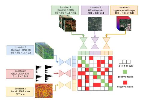
Figure 6.2: **Cross-Modal Contrastive Learning.** We consider a set of encoders for different inputs: image time series, LiDAR scans, hyperspectral images, etc. Each multi-modal patch is embedded by a dedicated encoder into a small  $5 \times 5$  feature map of width 128, whose cells are trained to be co-linear with the corresponding cell in the same modality and contrasted with others.
