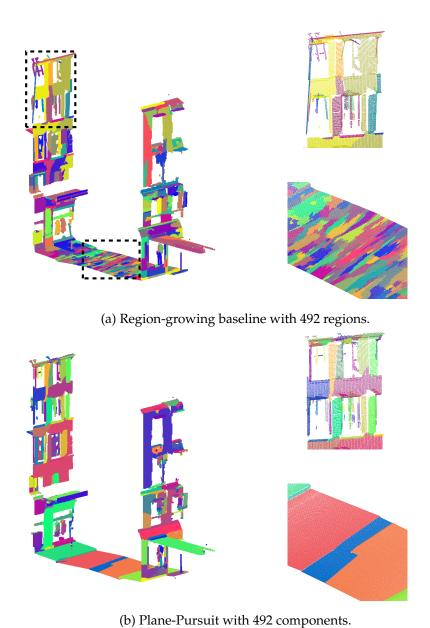
Figure 2.8: **Qualitative Results for Plane-Pursuit.** We represent the projection of each point on their supporting plane, and each colour represents a different component/region. Our method yields planes of adaptive size: large in geometrically simple regions such as roads, and smaller for complex areas such as facades and window panes.
