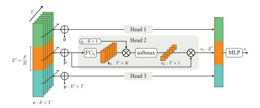
Figure 5.6: **L-TAE Architecture.** An input sequence **e** of T vectors of size E, with H=3 heads and keys of size K. The channels of the input embeddings are distributed among heads. Each head uses a learned query  $\hat{q}_h$ , while a linear layer  $FC_h$  maps inputs to keys. We concatenate the outputs of all heads into a vector the same size as the input embeddings.
