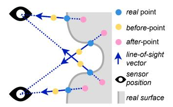
Figure 4.10: **Visibility-Augmented Point Cloud.** Each observed point is associated with a sightline unit vector pointing toward its sensor. New points are added before and after each point to help disambiguate occupancy.
