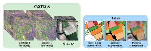
Figure 5.13: **MultiModal Dataset.** We introduce the PASTIS-R dataset containing 2433 multimodal image time series of Sentinel-2 optical and Sentinel-1 radar data. We evaluate different fusion strategies and enhancements on parcel-based classification, semantic segmentation, and panoptic segmentation.
