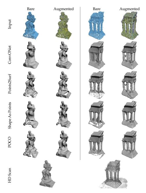
Figure 4.13: **Out-of-Domain Reconstruction.** Reconstructed shapes from a LiDAR point cloud (left, *Ignatius* from Tanks And Temples) and a MVS point cloud (right, *TempleRing* from Middlebury) using four different DSR methods trained on ModelNet10, with and without visibility information.
