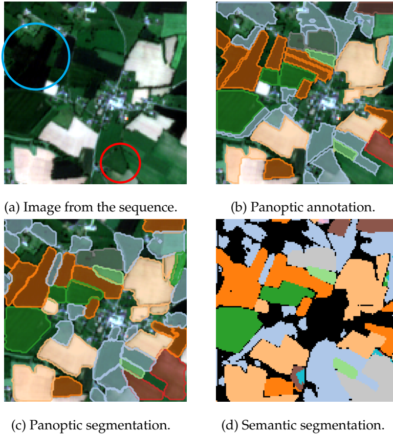
Figure 5.8: Problem Statement. We consider an image sequence (a) with panoptic annotations (b). Our objective is to learn spatio-temporal pixel features, which can be used to perform panoptic (c) and semantic segmentation (d). We observe some difficult configurations: boundary ambiguities that can not be resolved from a single image (cyan circle \circ ), and conversely, visually fragmented areas annotated as a single instance (red circle \circ ).
