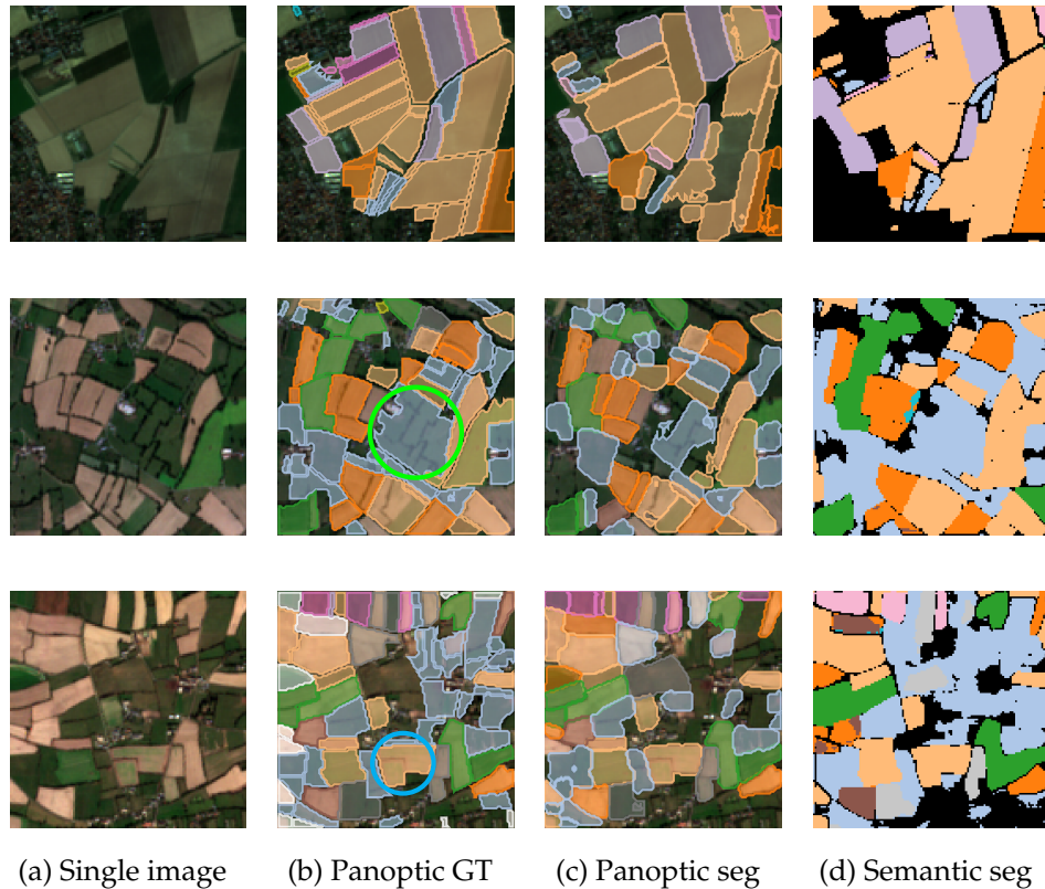
Figure 5.12: Qualitative Panoptic Segmentation Results. We present a single image from the sequence using the RGB channels (a), and whose ground truth parcel boundaries and types are known (b). We then present our predicted panoptic segmentation (c), and semantic segmentation (d). Large, fragmented parcels are sometimes declared as one single field \circ , making their recovery difficult. Conversely, fragmented parcels \circ are correctly predicted as a single instance, suggesting that our network is able to use the temporal dynamics to recover ambiguous borders.
