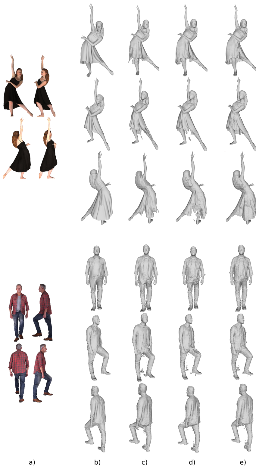
Figure 3.8: Ablation studies of our approach: a) Input cropped images. The 4 input images are rendered with the rotations around the vertical axis : 10^\circ , 110^\circ , 150^\circ , 300^\circ . b) Ground truth models. c) Ours without the attention-based view fusion module. d) Ours without the local 3D context encoding. e) Our full method.
