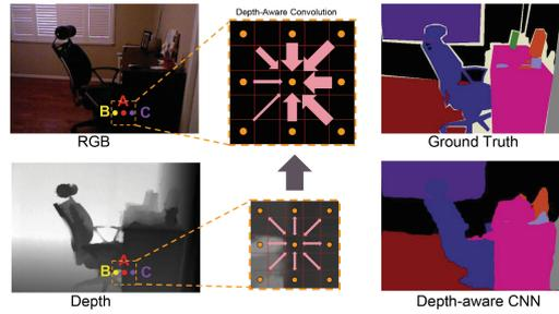
FIGURE 2.21: Illustration of depth-aware convolution. The image is from [154].
