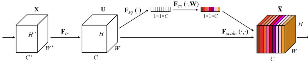
FIGURE 2.4: Illustration of SENet. The image is from [64]
