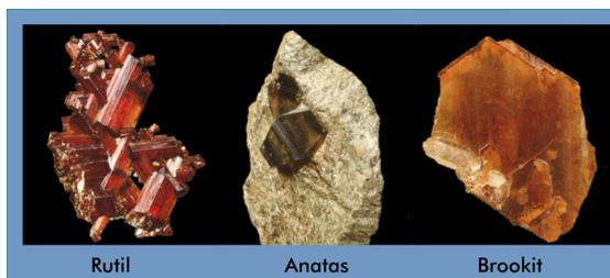
**Figure 1.15.** Three crystal forms of titanium dioxide in nature [111].
