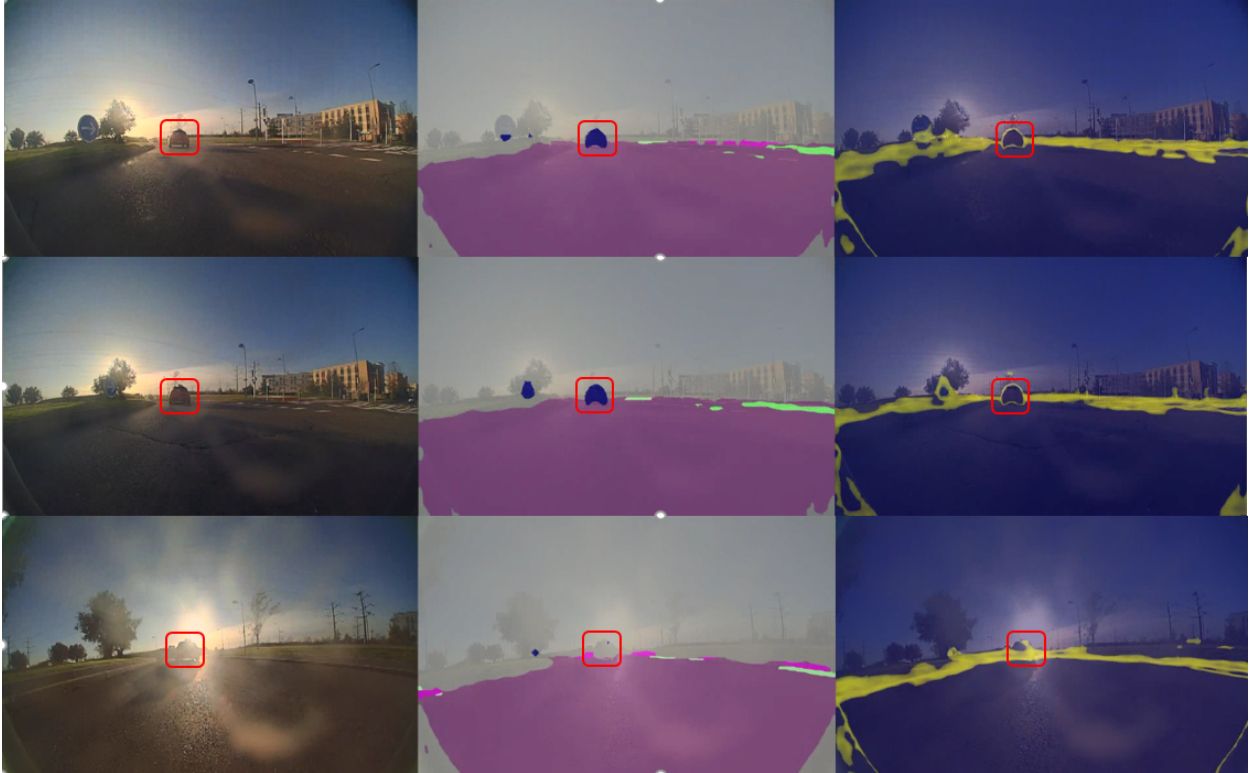
Figure 6.14: Online test: In this sequence, we show that our observer is able to detect a wrong prediction due to sun glare, in a live demo.
