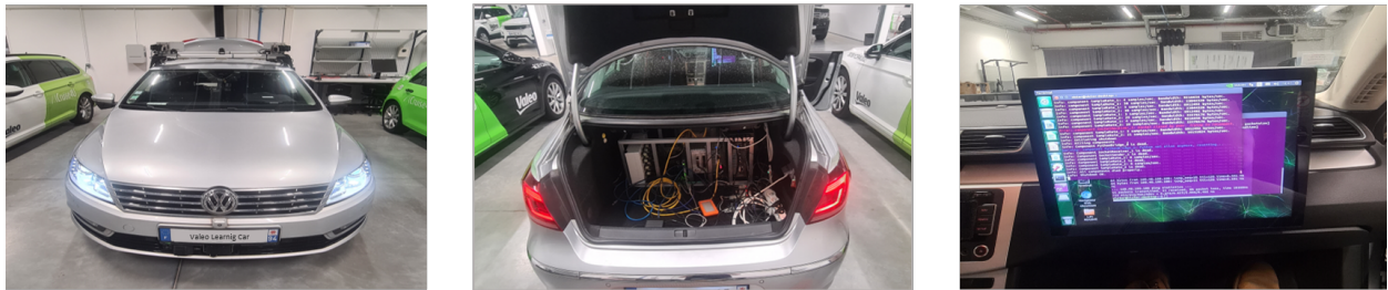
Figure 6.7: Car overview: On left the front view of the car, on the middle the back of the car with the Host PC and the Nvidia Jetson, and on the right the indoor monitor.
