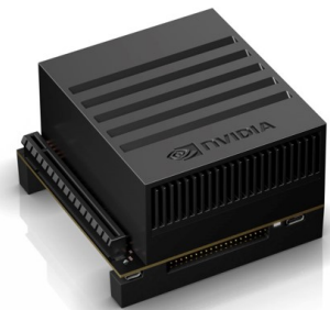
Figure 6.8: Nvidia Jetson Xavier: Hardware for accelerating ML applications.
