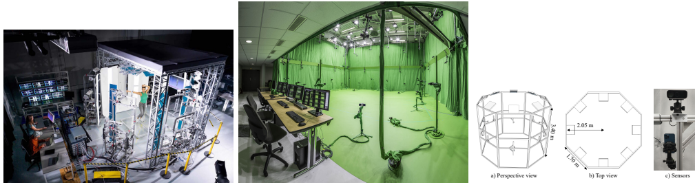
Figure 1.3 Different type of 4D acquisition systems: 4D Scanner at MPI Tübingen, Kinovis multi-view 4D acquisition room, Shanghai artificial laboratory 4D multi-view acquisition system
