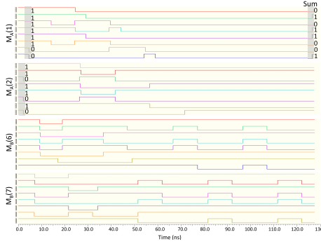
Fig. 14. Transient simulation for the in-memory 8-bit addition process.
