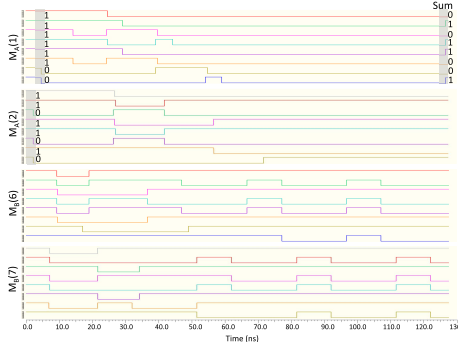
Fig. 14. Transient simulation for the in-memory 8-bit addition process.
