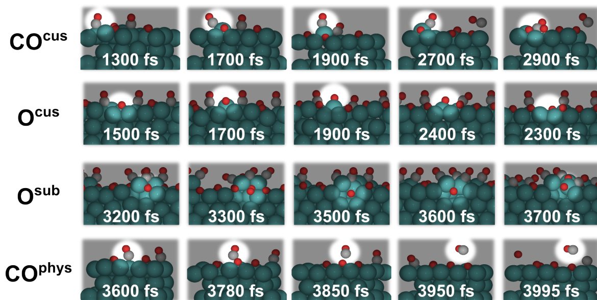
Figure 5.9: Snapshots of (T_e, T_{ph}) -AIMDEF simulations at low surface coverage in which different species of interest are formed. Each row of snapshots is devoted to the formation of the species named at the left. Each snapshot is labeled with the time step to which it corresponds. The area of interest for the formation of the species is enlightened making darker the rest of the snapshot. The central panel in each row corresponds to the time step in which the specific species is formed.
