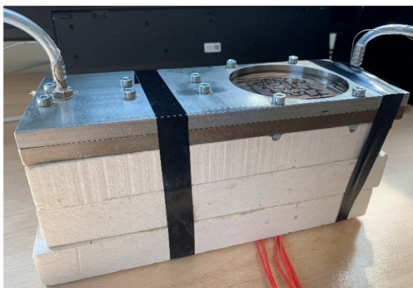
Figure 5.12 The insulation of the test section for the thermal test.
