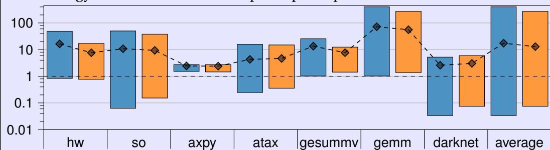
Figure 5.12.: Scenario NVM (1): Best, worst and average (♦) of all cases for both energy reduction (blue) and speedup (orange) normalized against SIMD reference (higher is better)
