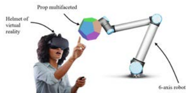
Fig. 3. Conceptual scheme of the experimental platform
