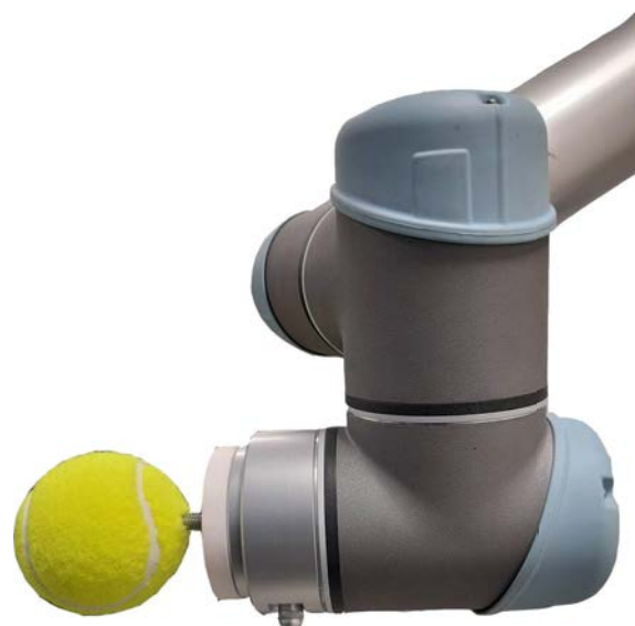
Figure 1. The designed prop, a physical representation of the virtual objects presented to the user during interaction.
