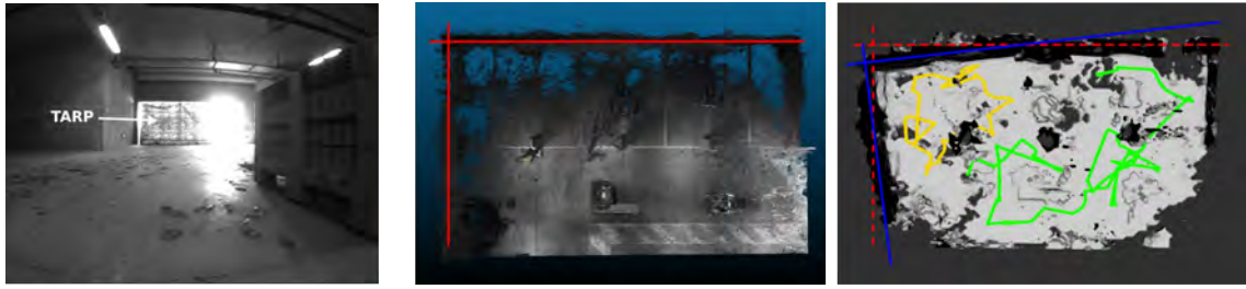
Figure 5.4: Some causes and consequences of the odometry drift. [left] Picture from left camera of the stereo-rig with the presence of a light halo at the parking lot entrance, partly covered by a tarp. [center] Top view of the ground truth of the parking lot with right angle corner formed by the walls (red lines). [right] Example of a consequence of the drift on the reconstruction: expected (red) vs. reality (blue).
