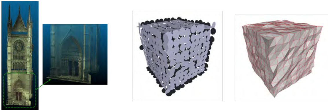
Figure 1.1: Surface shape representation: [left] Point cloud of the South portal of Amiens Cathedral; [middle] Examples of a surfel model and [right] a triangular surface mesh of a cube from [Andersen et al. 2010].
