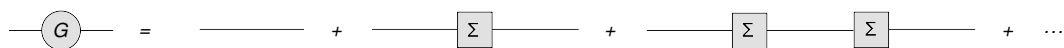
Figure 3.1: Usual diagrammatic interpretation of the Schwinger-Dyson equations for the two-point function G . The self-energy \Sigma is a sum of 1PI two-point diagrams. On the right-hand side, each line represents a free propagator G_0 .
