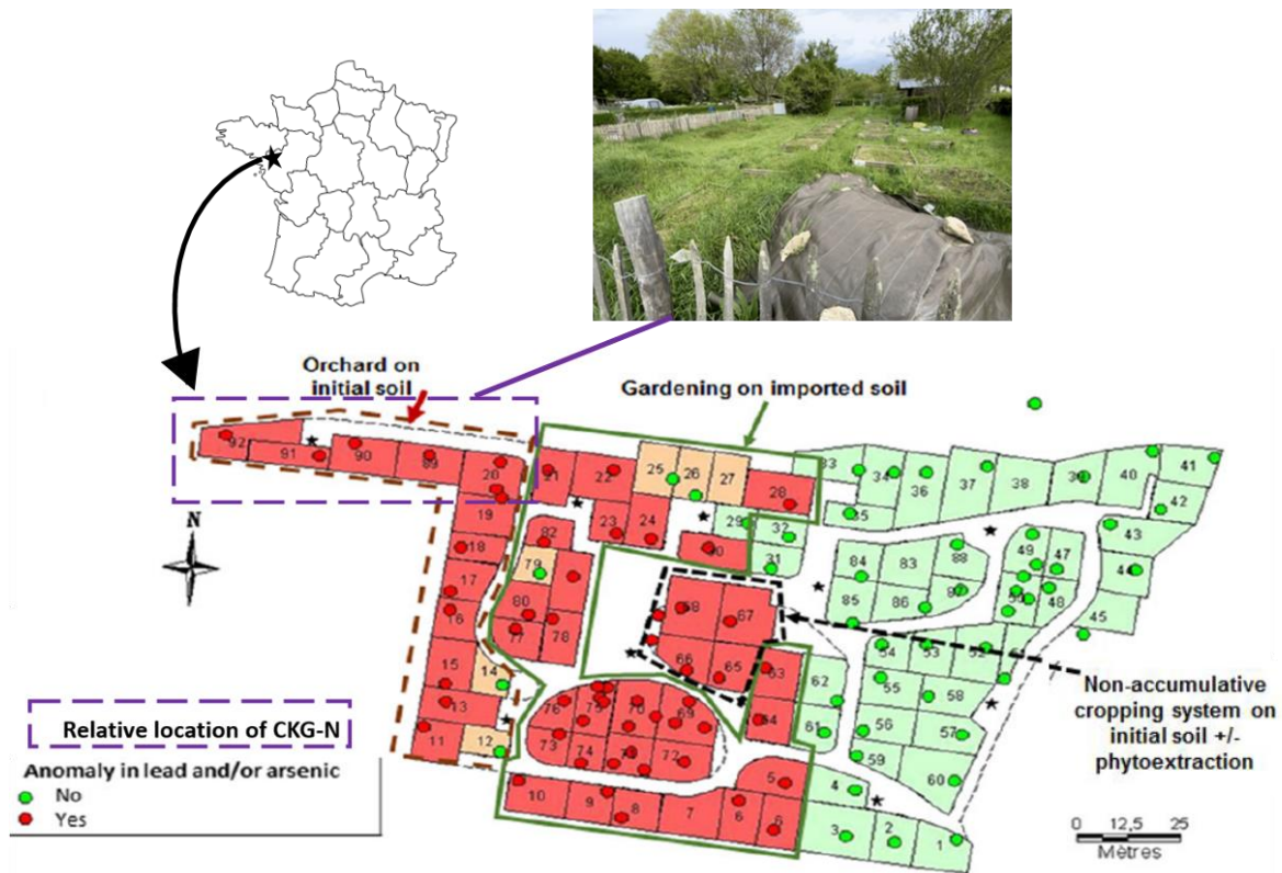
Figure 2-3: CKG-N localization in Les Eglantiers community kitchen garden (Nantes, France) and mapping of anomalies in Pb and As concentrations in the first 25 cm of soil exceeding background values (adapted from Le Guern et al., 2018)
