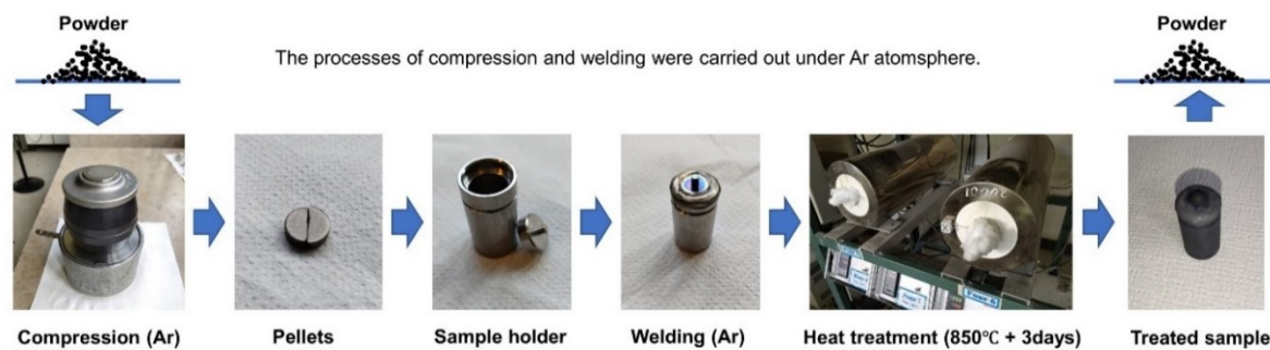
Figure 3.3 The procedure of sample preparation for heat treatment in ICMPE.
