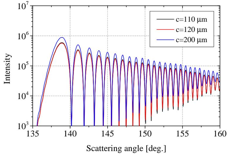
Figure 5.13 – The scattering diagrams of three prolate ellipsoids for the perpendicular polarization. The axes of the ellipsoid are  $a = b = 100 \mu\text{m}$ , and  $c = 110 \mu\text{m}$ ,  $c = 120 \mu\text{m}$  and  $c = 200 \mu\text{m}$ . The refractive index is  $m = 1.333$ . The wavelength the incident plane wave is  $\lambda = 0.6328 \mu\text{m}$ .
