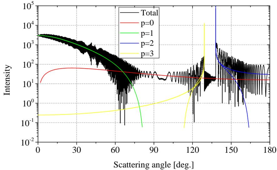
Figure 2.10 – Scattering diagrams of an infinite circular cylinder. The incident plane wave with wavelength  $\lambda = 0.6328 \mu\text{m}$  is in perpendicular polarization. The radius of particle and its refractive index are  $a = 100 \mu\text{m}$  and  $m = 1.333$ .
