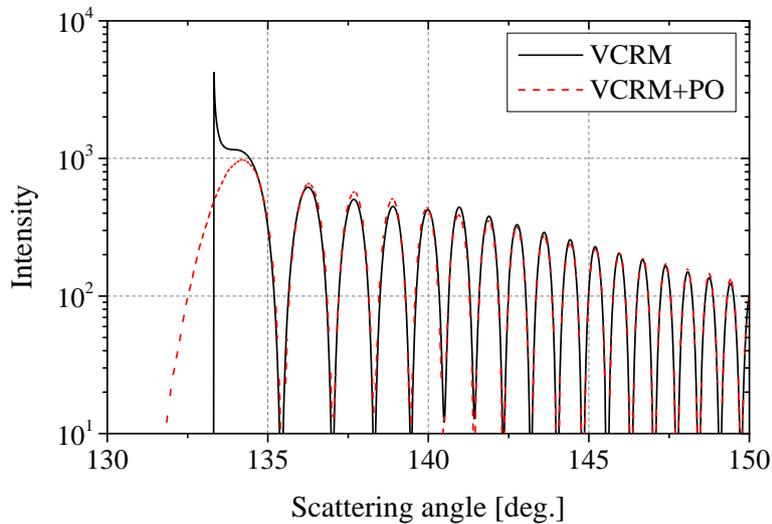
Figure 5.6 – Scatting diagrams of an infinite elliptical cylinder near rainbow region with particle size in  $a = 95 \mu\text{m}$ ,  $b = 100 \mu\text{m}$  and wave in perpendicular polarization for  $p = 2$ .
