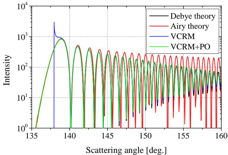
Figure 4.9 – Scattering diagrams of the primary rainbow of an infinite circular cylinder of refractive index  $m = 1.333$  and radius  $a = 100 \mu\text{m}$ . The incident plane wave  $\lambda = 0.6328 \mu\text{m}$  is normal to the cylinder and polarized perpendicular to the scattering plane.
