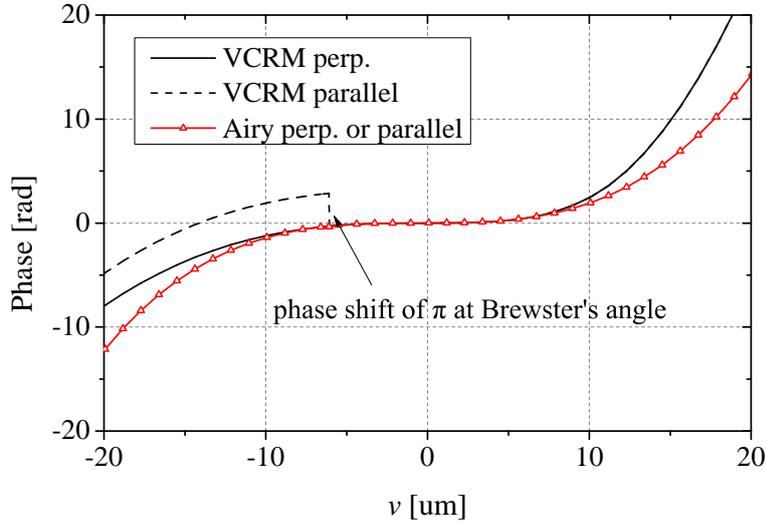
Figure 4.5 – Phase on the virtual line of  $p = 2$ . The polarization of the incident wave ( $\lambda = 0.6328 \mu\text{m}$ ) is perpendicular to the scattering plane. The radius of the particle is  $a = 100 \mu\text{m}$  and its relative refractive index  $m = 1.333$ .
