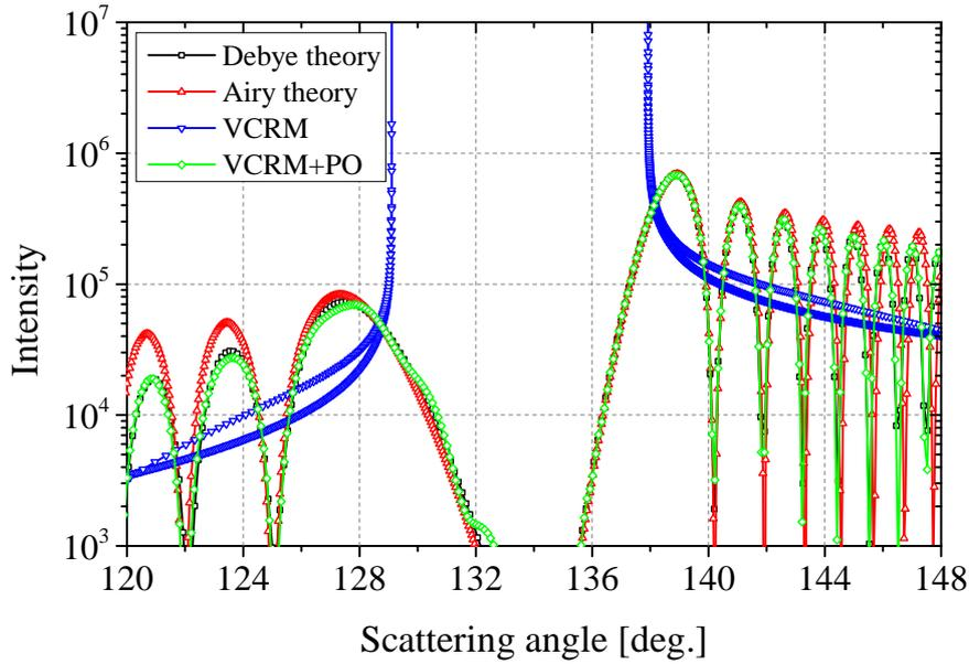
Figure 4.18 – Scattering diagrams of a sphere near the primary and secondary rainbows ( $p = 2, 3$ ) angle in perpendicular polarization. The incident wave is a plane wave of wavelength  $\lambda = 0.6328 \mu\text{m}$ . The particle size is  $a = 100 \mu\text{m}$  with refractive index  $m = 1.333$ .
