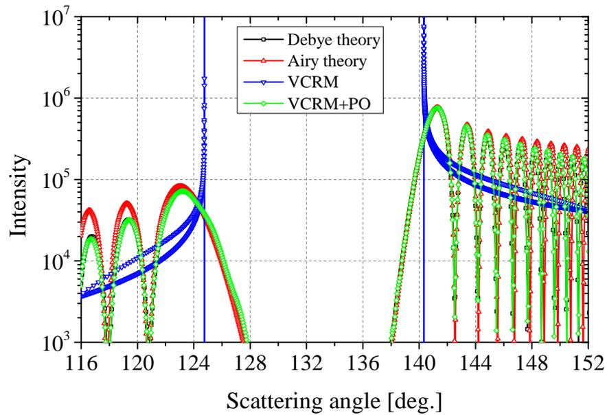
Figure 4.20 – Scattering diagrams of a sphere near the primary and secondary rainbows ( $p = 2, 3$ ) angle in perpendicular polarization. The incident wave is a plane wave of wavelength  $\lambda = 0.6328 \mu\text{m}$ . The particle size is  $a = 100 \mu\text{m}$  with refraction index  $m = 1.35$ .
