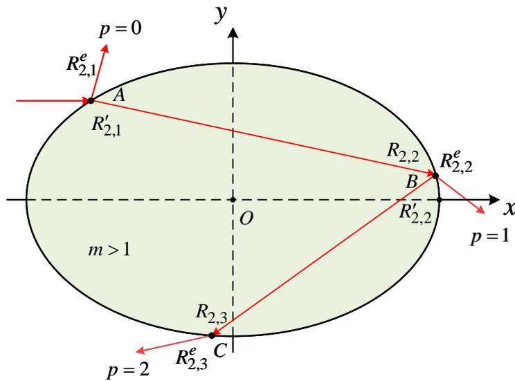
Figure 3.4 – Divergence factor in an elliptical cylinder.
