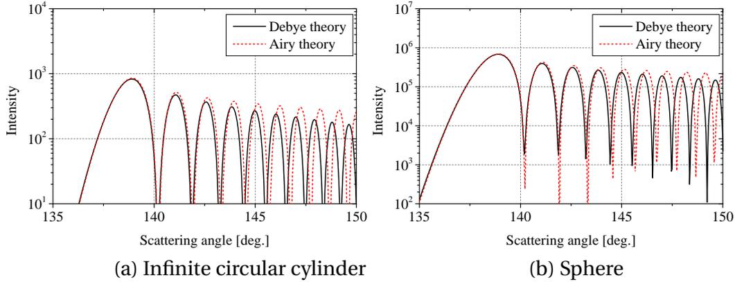
Figure 4.2 – Scattering diagrams of an infinite circle cylinder (left) and a sphere (right) of  $p = 2$  in the rainbow region. The polarization of the incident wave ( $\lambda = 0.6328 \mu\text{m}$ ) is perpendicular to the scattering plane. The radius of the particle is  $a = 100 \mu\text{m}$  and its relative refraction index  $m = 1.333$ .
