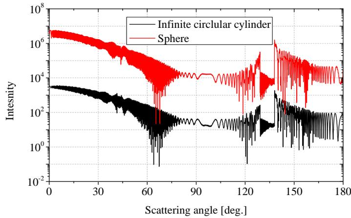
Figure 2.12 – Comparison the scattering diagrams of a sphere and infinite circular cylinder. The incident plane wave with wavelength  $\lambda = 0.6328 \mu\text{m}$  is in perpendicular polarization. The radius of particle and its refractive index are  $a = 100 \mu\text{m}$  and  $m = 1.333$ .
