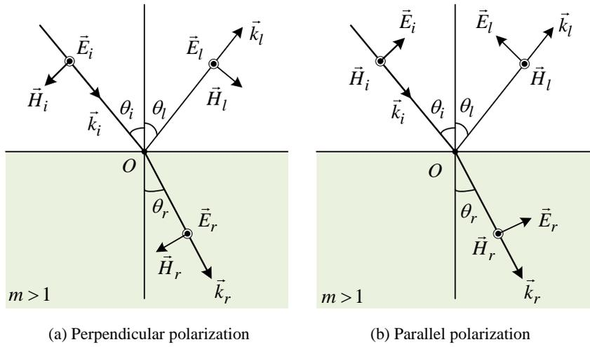
Figure 2.1 – Schema for derivation of Snell's law.
