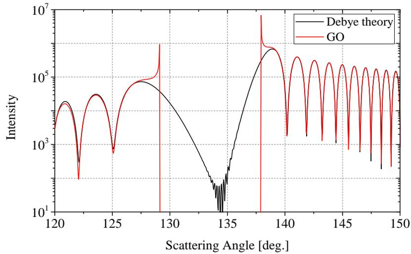
Figure 2.17 – Scattering diagrams of  $p = 2$  and  $p = 3$  for a sphere in perpendicular polarization by Debye theory and GO. The incident plane wave with wavelength  $\lambda = 0.6328 \mu\text{m}$  is in perpendicular polarization. The radius of particle and its refractive index are  $a = 100 \mu\text{m}$  and  $m = 1.333$ .
