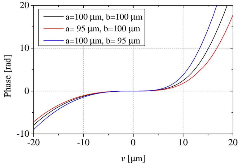
Figure 5.2 – Phase the rays  $p = 2$  on the virtual line of an elliptical cylinder illuminated by a plane wave of wavelength  $\lambda = 0.6328 \mu\text{m}$  in perpendicular polarization. The relative refraction index of the particle is  $m = 1.333$ .
