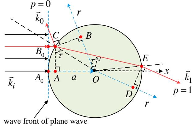
Figure 2.9 – Phase due to the optical path.
