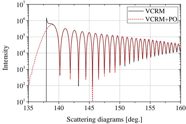
Figure 5.11 – The scattering diagrams of three prolate ellipsoid in the perpendicular polarization. The axes of the ellipsoid are  $a = b = 100 \mu\text{m}$ , and  $c = 120 \mu\text{m}$ . The refractive index is  $m = 1.333$ . The wavelength the incident plane wave is  $\lambda = 0.6328 \mu\text{m}$ .
