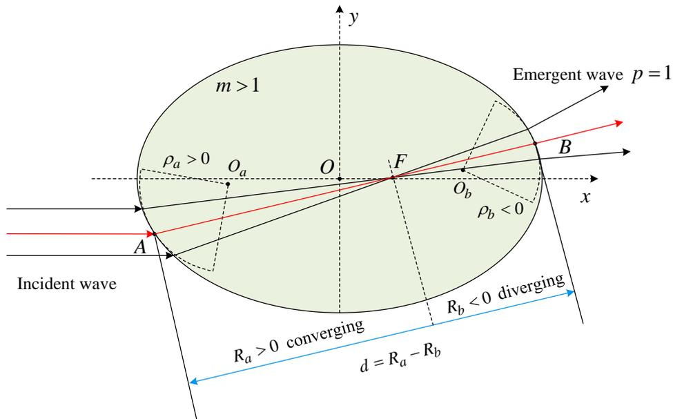
Figure 3.1 – Convention the sign of curvature radii.
