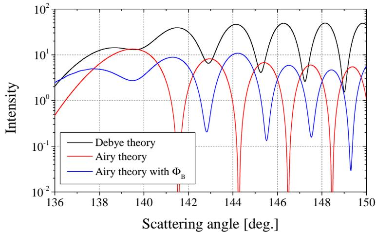
Figure A.2 – Comparison of the scattering diagrams in the neighborhood of the primary rainbow ( $p = 2$ ) with the parallel polarization calculated by the Debye theory, the Airy theory and the the Airy theory with phase jump. The particle is an infinite circular cylinder of radius  $a = 50 \mu\text{m}$ , refractive index  $m = 1.333$  illuminated normally by a plane wave of wavelength  $\lambda = 0.6328 \mu\text{m}$ .
