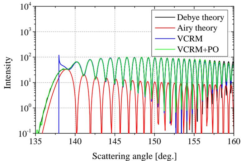
Figure 4.12 – Scattering diagrams of the primary rainbow of an infinite circular cylinder of refractive index  $m = 1.333$  and radius  $a = 100 \mu\text{m}$ . The incident plane wave  $\lambda = 0.6328 \mu\text{m}$  is normal to the cylinder and polarized parallel to the scattering plane (along the axis of the cylinder).
