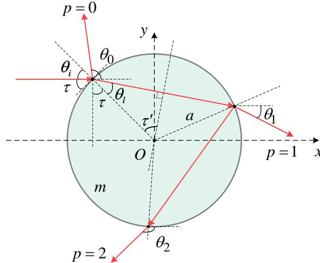
Figure 2.7 – Optical path in a circular cylinder.
