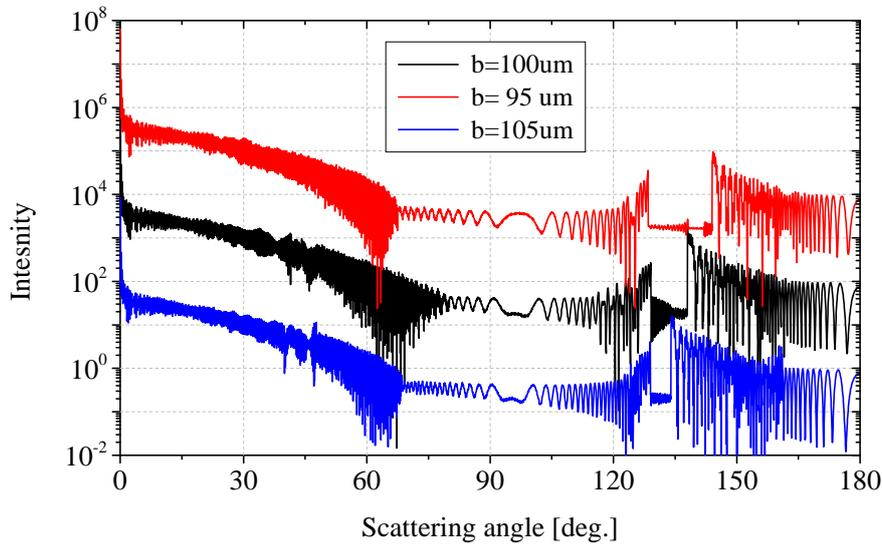
Figure 3.7 – Scattering diagrams of an infinite elliptical cylinder. The incident wavelength is  $0.6328 \mu\text{m}$  and in perpendicular polarization. The other parameters of the particles are  $a = 100 \mu\text{m}$  and the relative refraction index  $m = 1.333$ . For clarity, the scattering diagrams are offset by  $10^{-2}$  and  $10^2$ .
