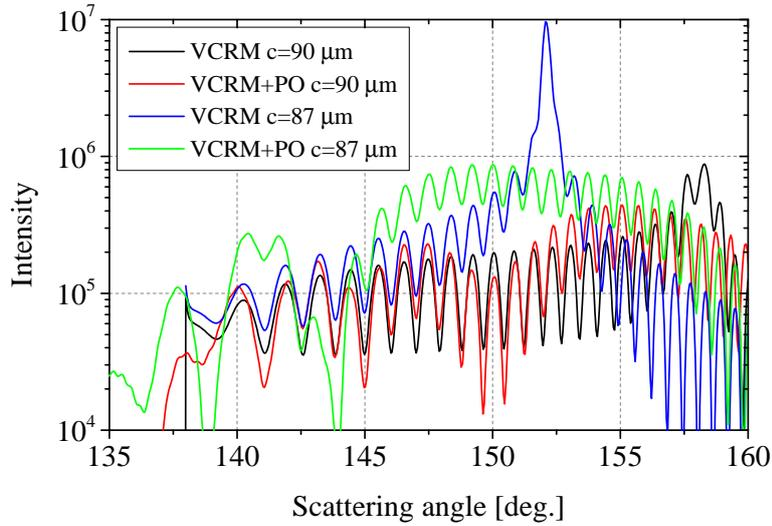
Figure 5.18 – The scattering field of an oblate spheroid in parallel polarization near rainbow region. Same other parameters as in Figure 5.17.
