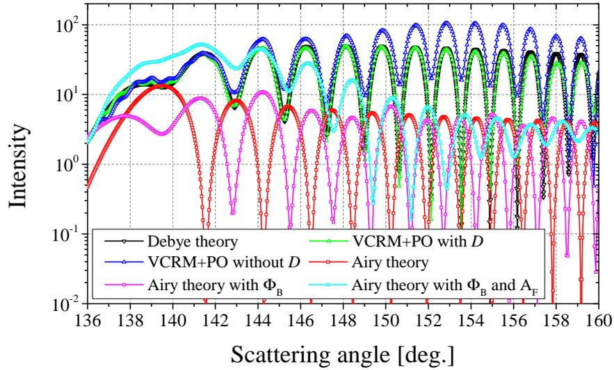
Figure 4.17 – Scattering diagrams of a circular cylinder near the primary rainbow angle in parallel polarization. The incident wave is a plane wave of wavelength with  $\lambda = 0.6328 \mu\text{m}$ . The particle size is  $a = 50 \mu\text{m}$  with refraction index  $m = 1.333$ .
