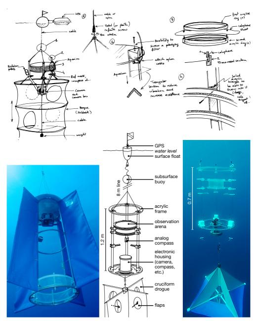
**Figure 2.4:** Several iterations on the design of the DISC instrument. Bottom left: first prototype with aluminium frame, integrated drogue and a downward pointing video camera. Top: my drawings for a circular, acrylic-based design with a separate holey-sock type drogue. Bottom centre: final version of the circular design with a DSLR camera housing. Bottom right: current smaller version of the instrument with a GoPro camera and a star-shaped drogue.
