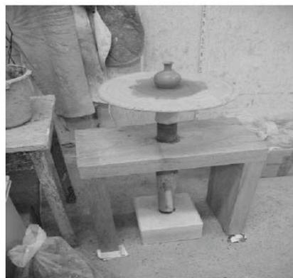
Fig. 1: Experimental LM potter's wheel built on the flat to pot in a seated position.
