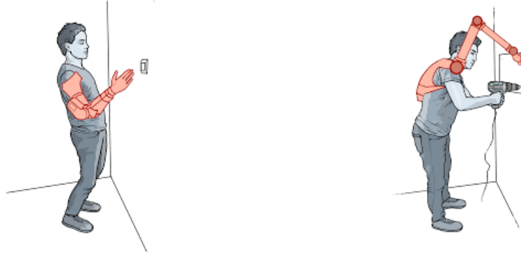
(a) Subject leans backward to create an upward motion at the end-effector of the prosthetic arm. (b) Subject leans forward to create forward motion at the end-effector of the supernumerary arm.
