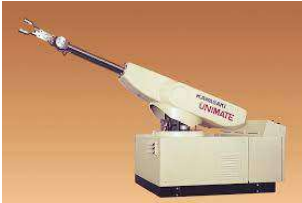
(a) Unimate by Unimation is considered the first industrial robot in history. This robot, hydraulically actuated, was installed in the General Motors factory.
