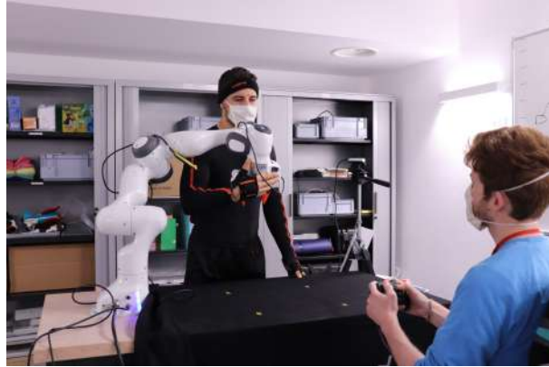
Figure 3.10: Set-up for EXP2 : the robot executes pseudo-random movements while it is controlled by a second operator using a joystick.
