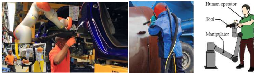
(a) Human-Robot comanipulation in Industry (b) Robotic co-worker for industrial abrasive blasting [44].
