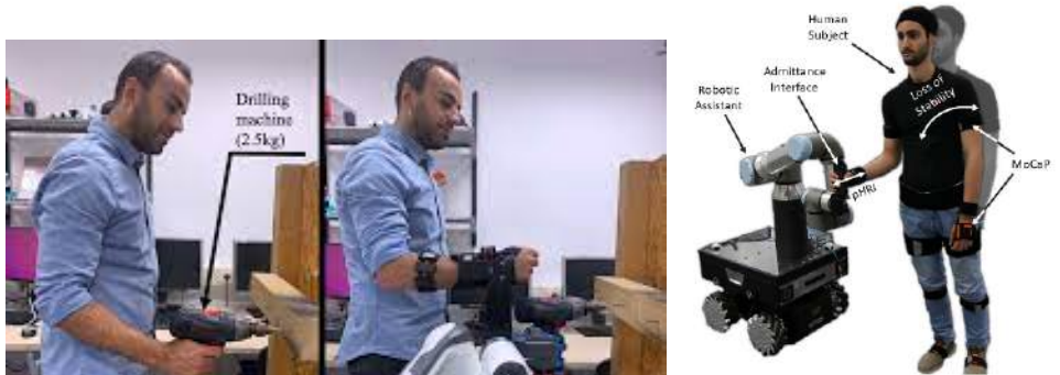
(e) Collaborative screwing using MOCA-MAN [111] (f) Kairos platform helping Improving Standing Balance for human [193]
