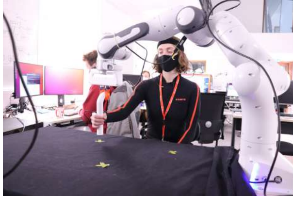
Figure 3.12: Set-up for EXP3 : Human and robot are coupled, the robot executes the same trajectory ten times while the human follows its movements.
