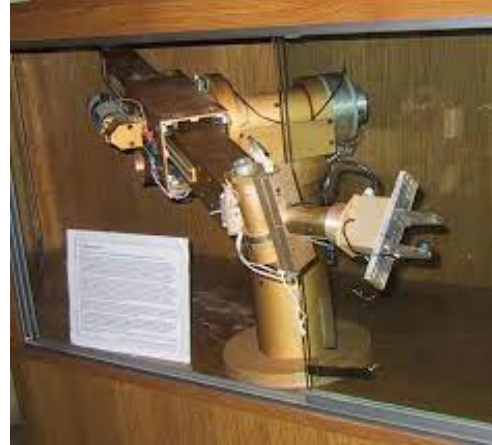
(b) Stanford Arm: the first prototype of a robot actuated by electric motors and controlled by a microprocessor.
