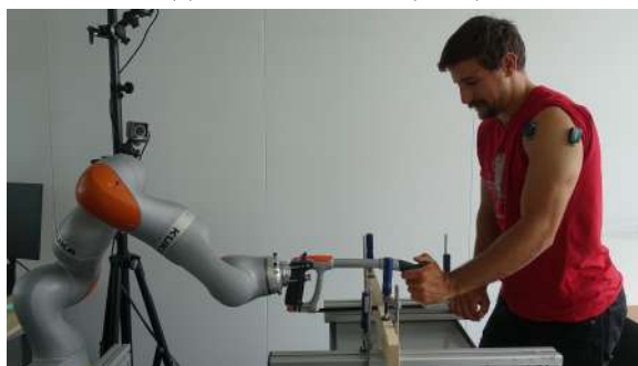
(e) The LBR iiwa released in 2014 by KUKA. LBR stands for “Leichtbauroboter” (German for lightweight robot), iiwa for “intelligent industrial work assistant”.
