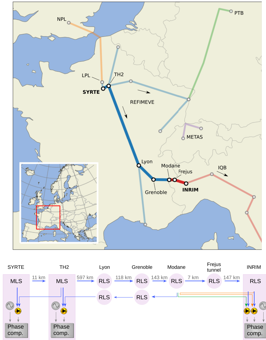
FIG. 1. Geographical layout of the infrastructure, with the link between SYRTE, Paris (France) and INRIM, Torino (Italy) characterized in this work highlighted as a thick line. The map also shows the other branches of the REFIMEVE network in blue and the Italian Quantum Backbone (IQB) in red. Cross-border connections of this infrastructure to the National Metrology Institutes NPL in the UK and PTB in Germany are indicated in orange and green. Repeater laser stations (RLS or MLS) and link terminals are represented with open circles. (b) The scheme used for the link characterization: blue paths indicate phase-stabilized links on the two fibers. At SYRTE, local reference light is sent to a photodiode together with the light disseminated through the loop SYRTE-TH2-SYRTE and phase compared to a local rf reference, to evaluate the overall uncertainty of the SYRTE-TH2-SYRTE link (similarly for the path to Modane). The green arrow represents a free-running link whose noise is removed offline. This is detected by heterodyning local radiation at INRIM with light traveling the path INRIM-Modane-INRIM (orange line). The Modane-INRIM link is evaluated by comparing light disseminated through the two fibers.
