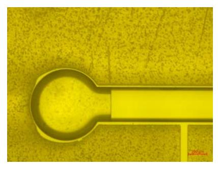
**Figure 4.8:** Picture of the glass substrate after channel engraving and enduction, development lithography steps.
