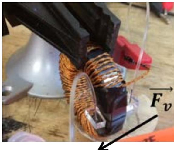
**Figure 4.3:** Picture of the setup composed of the microfluidic chip with an inset and outlet of solution inserted in the gap of a magnetic core with ferrite.
