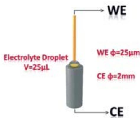
**Figure 2.7:** Schematic representation (not to scale) of the conventional working UME ( $\phi = 25 \mu\text{m}$ ) dipping into  $\text{Fe}^{II}/\text{Fe}^{III}$  and methylene blue (MB) electrolyte on top of the counter electrode ( $\phi = 2 \text{ mm}$ ).
