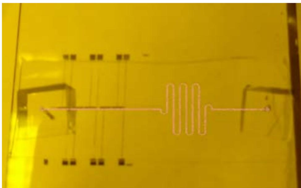
**Figure 4.10:** Picture of the final PDMS/glass microfluidic setup for magnetic hyperthermia and electrochemical detection coupling. Microfluidic channel is colored in lightred.
