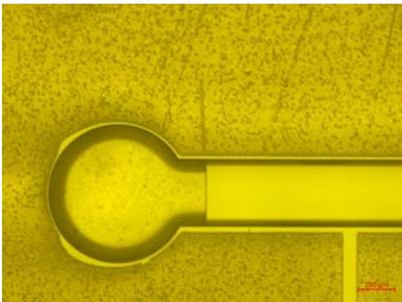
**Figure 4.8:** Picture of the glass substrate after channel engraving and enduction, development lithography steps.
