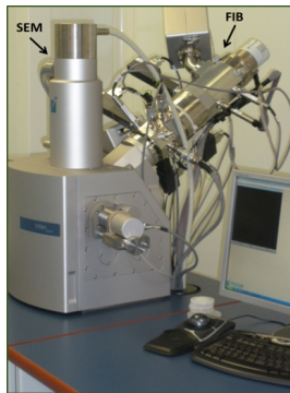
Figure A.21: a dual beam Tescan LYRA1 XMH FIB SEM instrument.
