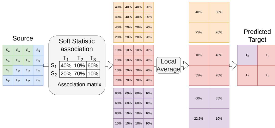
Figure 4.4: SoftMaxProba : the translated class is obtained by averaging the probability of each source class to correspond to each target class and choosing the most probable one.
